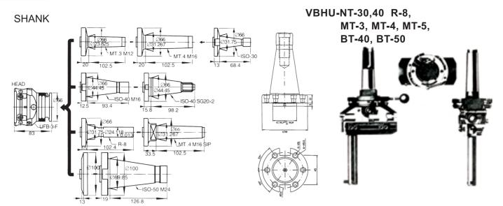
Main part of the universal boring heads is the body(1), in which the tool slide (3) moves on dovetail guideways. The tool slide is provided with holes for accommodation of tools and tool holders(4). In boring holes or turning extenal cylindrical surfaces, the tool is adjusted with the aid of the graduated dial for fine setting of tool slide(5), one division of which means a change in diameter of bored hole by .0005".
